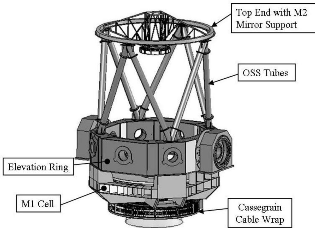
Figure 2 - DCT Optics Support Structure with RC Configuration
