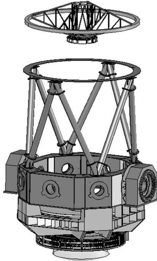
Figure 3 - Removable Top Ring for DCT Secondary
