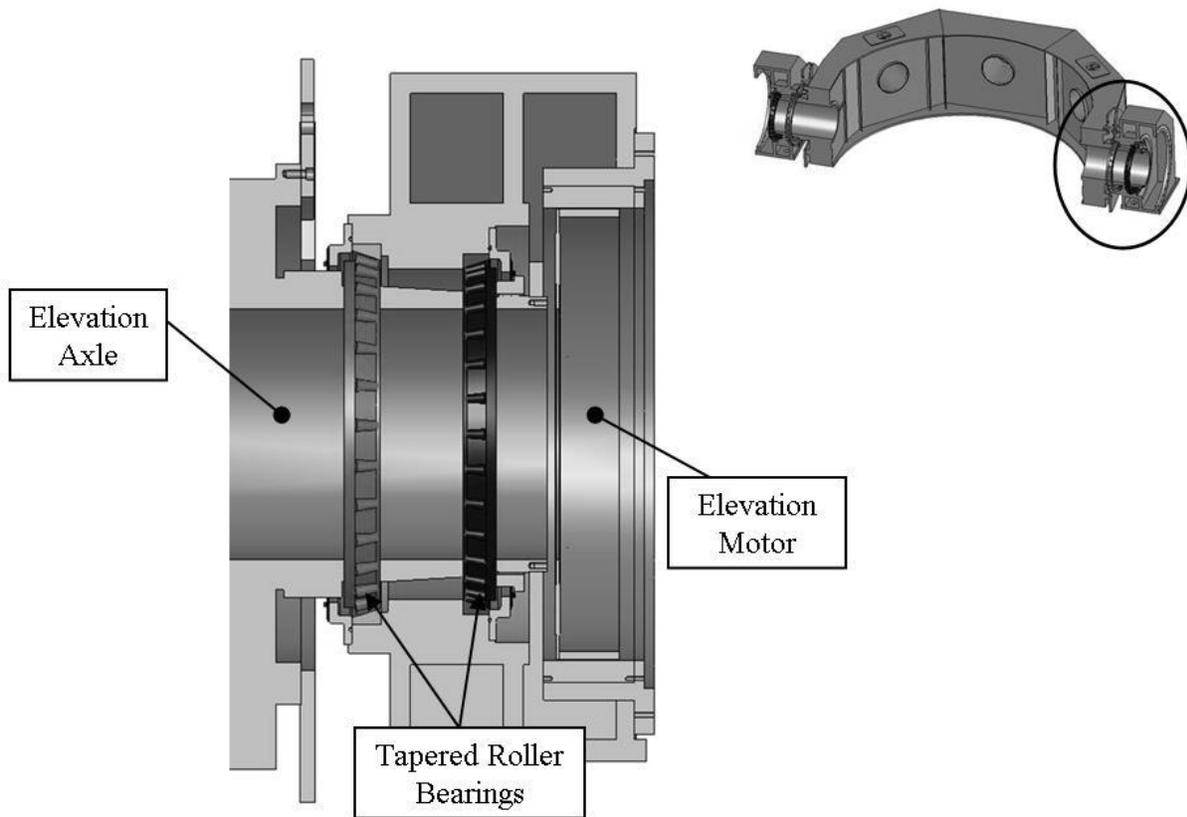
Figure 5 - DCT elevation drive
